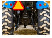
*High Capacity Three Point Hitch* Heavy-Duty Frame And Lift Cylinders Enable Three-Point
