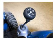
*Integrated Joystick* Provides Comfortable Access For Loader Operations. 3<sup>rd</sup> Function (Option)
