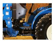
Rubber Platform **Matting And Step** Provide Added Comfort And Access To The Spacious Operator's Platform
