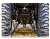
High Capacity Three Point Lifts Up To 1,808 lbs.
