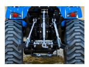
**Durability And Capacity** Heavy-Duty Frame And Lift Cylinders Enable 970 lbs. Of Three-Point Lift Capacity
