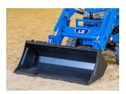
High Capacity Loader 2 Large Diameter Lift And 2 Large Diameter Curl Cylinders Enable 966 lbs. Lift Capacity
